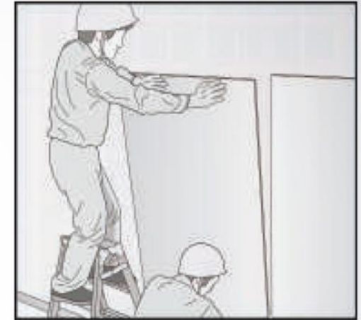
STEP 4. Pasting and crimping
